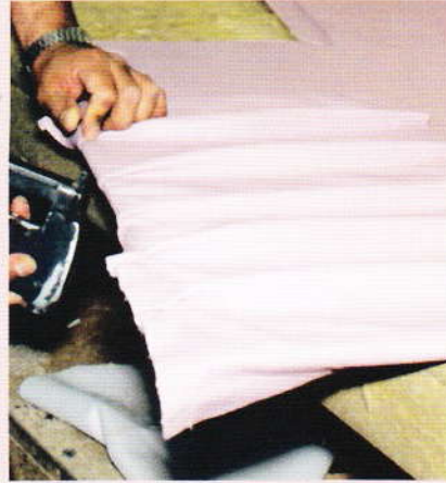
Photo 18. The project is finished by stapling the two sides to the big panel. Be careful stapling the bottom of the pleats to be sure they retain their correct shape and position.
