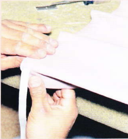
Photo 17. This is the exit area of the elastic. Frank will pull it snug then staple it to the panel. Don't make the elastic too tight. It will overstretch when the pocket is opened and tear away from the panel.
