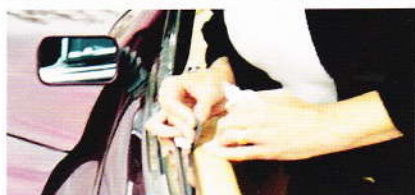
Photos 2 & 3. The process turns out to be very simple. On the very small scratches she applies a drop or two of instant glue. Next, with 400-grit wet-or-dry sand paper, she gently sands over the scratch and glue. This closes the scratch and sands away any fibers or bits of material left standing. It works with both leather and vinyl.
